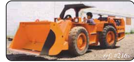
ref. #216s JCI 125, Deutz F4L912W, powershift transmission, ROPS canopy, fire suppression, ejector bucket, hydraulic disc brakes.... For more information call Mark Allen at Driftech Inc. 705-566-4384, fax: 705-560-8277, e-mail: mallen@driftech.com
