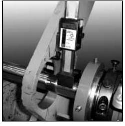
The Digital Bore Measuring Tool is compatible with all Climax boring machines with bars up to 2 inches in diameter. It presets to the bar diameters that the operator inputs. Once set, the tool determines the dimension from the center of the bar to the tip of the tool bit or the inside of the bore, allowing the diameter to be read and the cut to be finished.
